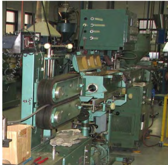
Figure 2: Extrusion system for production of profiles
