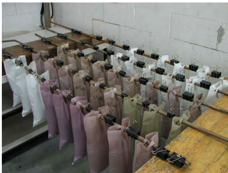
Figure 6 : APPARATUS USED TO SUSPEND BAGS FILLED WITH WATER
